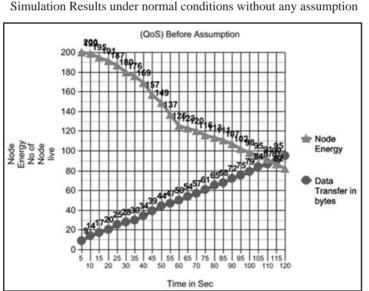
Graph 1 Simulation Results under normal conditions without any assumption
